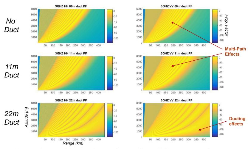
Propagation models must be used to predict to fully capture performance
