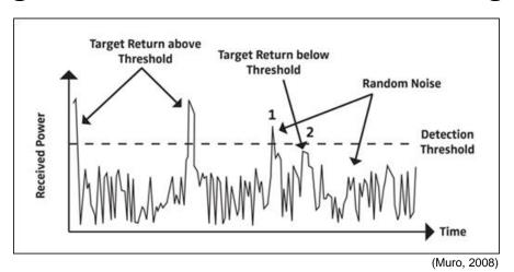
S/N is set to minimize false detections while ensuring enough signal is present to detect the target.
